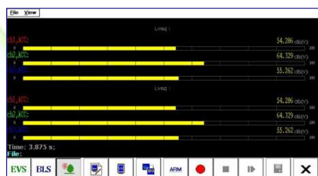
3-axis Human Response Vibration mode by JIS C 1510
